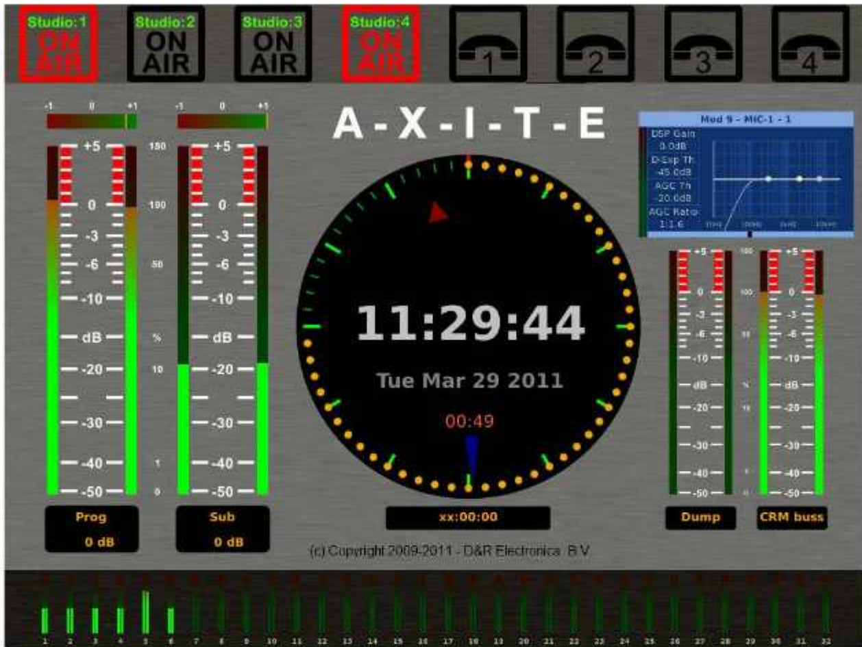
AXITE meter screen, that can directly be seen when you connect a HDMI connector to the control surface
