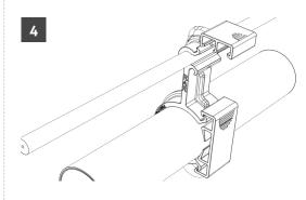
Insert rope into smaller RAR housing.
