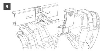
Insert cable into RAX clamp contrasting from below.
