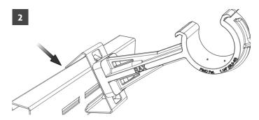
Hook upper clip-on corner on section, with cable clamp's opening facing upwards.
