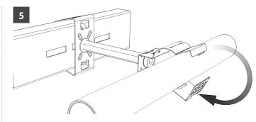
Insert the cable in the **SCC** and close the clamp.
